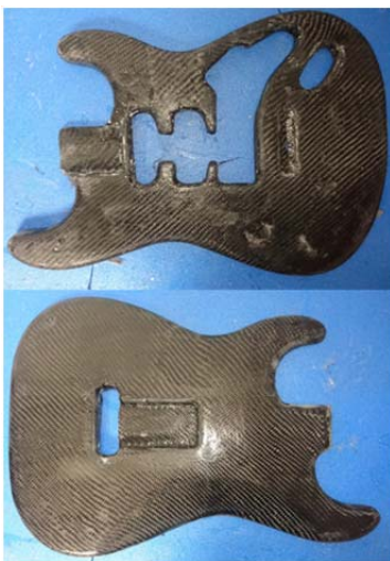
Figure 9. Modified parts removed from the mould
