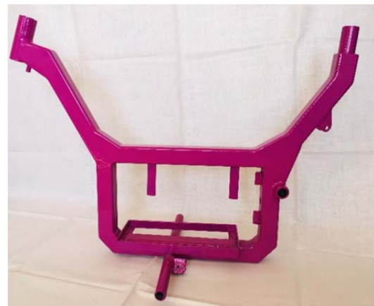
Figure 19. Finished frame of the electric motorcycle
